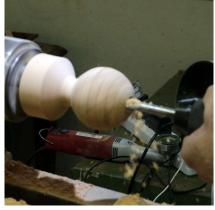
The next step is to hollow the globe. Drill a 3/8" hole all the way through. Use  $\frac{1}{2}$  or  $\frac{3}{4}$  inch drill leave  $\frac{1}{4}$ " at the bottom.
