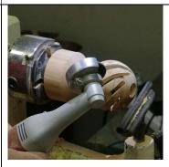
When you are finished hollowing use the rasp or mini sidegrinder to even out the thickness of the bines.
