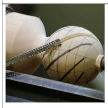
The cuts can be widened with a rasp or a surform tool shown here.
