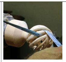
To round the bottom of the bines and smooth off the top use a cloth-backed sanding strip with a shoe-shine type motion.
