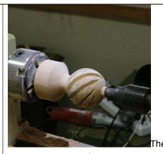
next step is to cut the spaces between the bines. The bines being the spiral parts that are left. It may seem strange to be doing this before hollowing, but it is better to do it while the cuts are supported by the solid sphere of wood.
