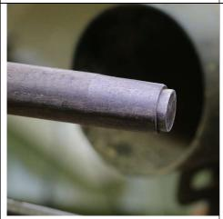
Starting with the top finial, turn a ¾" tenon to fit into the globe
