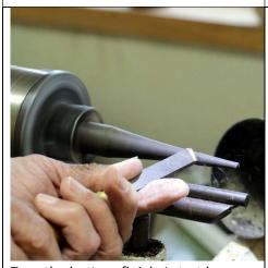
Turn the bottom finial. I start by tapering the blank from the headstock toward the tail stock.
