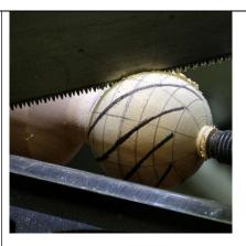
One way to do this is to use a saw to cut along the spiral lines, trying to get an even depth of cut along the surface.
