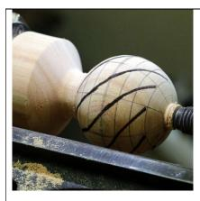
Shape the sphere and draw grid and cut lines. Notice that I have gone over one line horizontally and up two lines verically. The number of vertical lines determine the number of bines.
