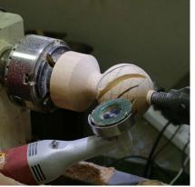
Another way to cut the groves is with a mini grinder and carbide disk cutter. This makes a groove about 1/8 to 3/16ths of an inch wide ¼" deep.
