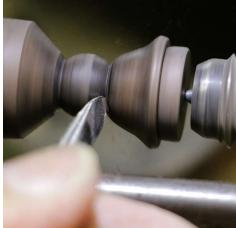
Turn the top finial to the desired shape – here I am using a detail gouge.
