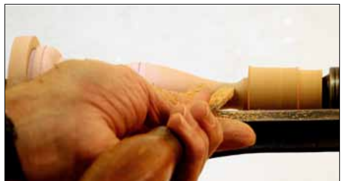
19 The bulb section ends with a cove that meets the fillet beneath the cup. Cut from the fillet down to the center of the cove, then smooth it off from the bulb side.
