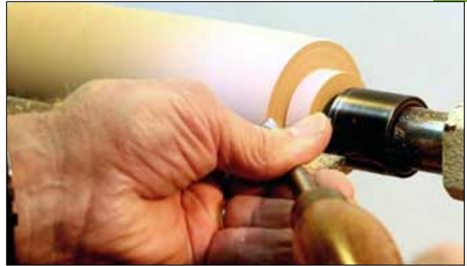
12 Face off the end using a small spindle gouge. Hold the tool level, rotate to the closed-flute position, and aim the bevel.
