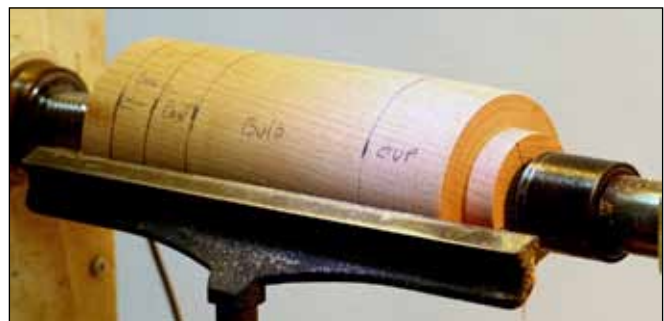
14 Mark the bottom of the cup, bottom of the bulb, bottom of small base, and bottom of large base.
