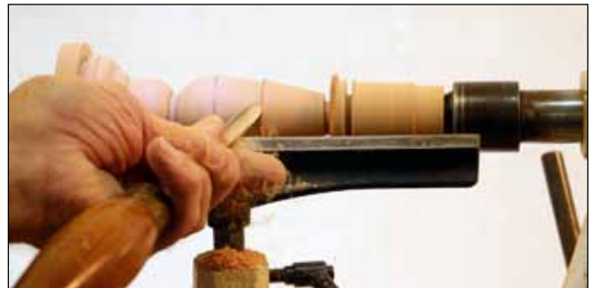
18 Work downhill both directions from the largest diameter line on the bulb section. Cutting to the right, the gouge handle angles downward and to the left, with the gouge flute rolling from fully open (12 o'clock) to closed (3 o'clock) at the end of the cut.
