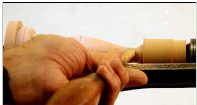
19 The bulb section ends with a cove that meets the fillet beneath the cup. Cut from the fillet down to the center of the cove, then smooth it off from the bulb side.
